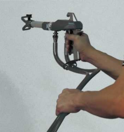
MIXED INSIDE THE MIX GUN
