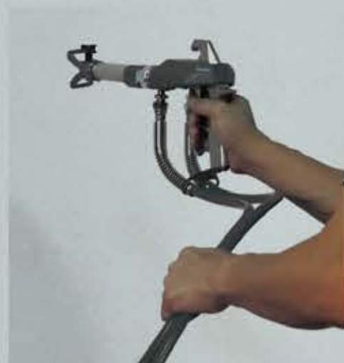
MIXED INSIDE THE MIX GUN
